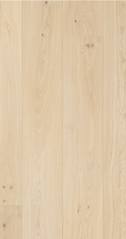
NATURAL A Knots: very few Cracks: none Sapwood: none
