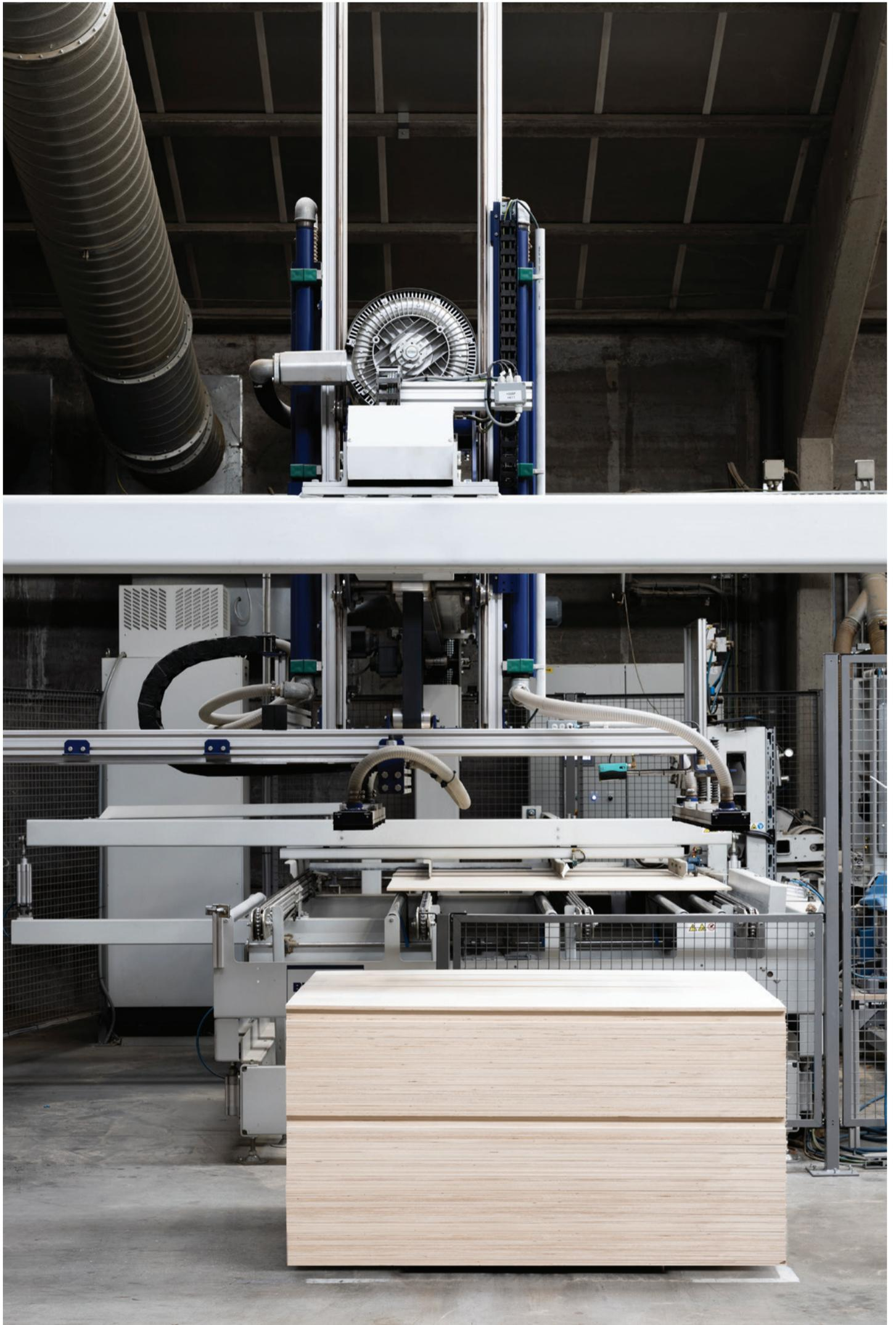
First, the sawn top layers are sorted by hand, after which they are glued to the plywood using a cold press technique. Belgiqia uses high-tech machines in the production process. This means we can guarantee a perfect fit. Afterwards, the boards are manually removed from the machines for an extra visual check.
